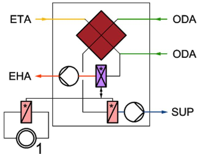
18. + air to air heat exchanger
