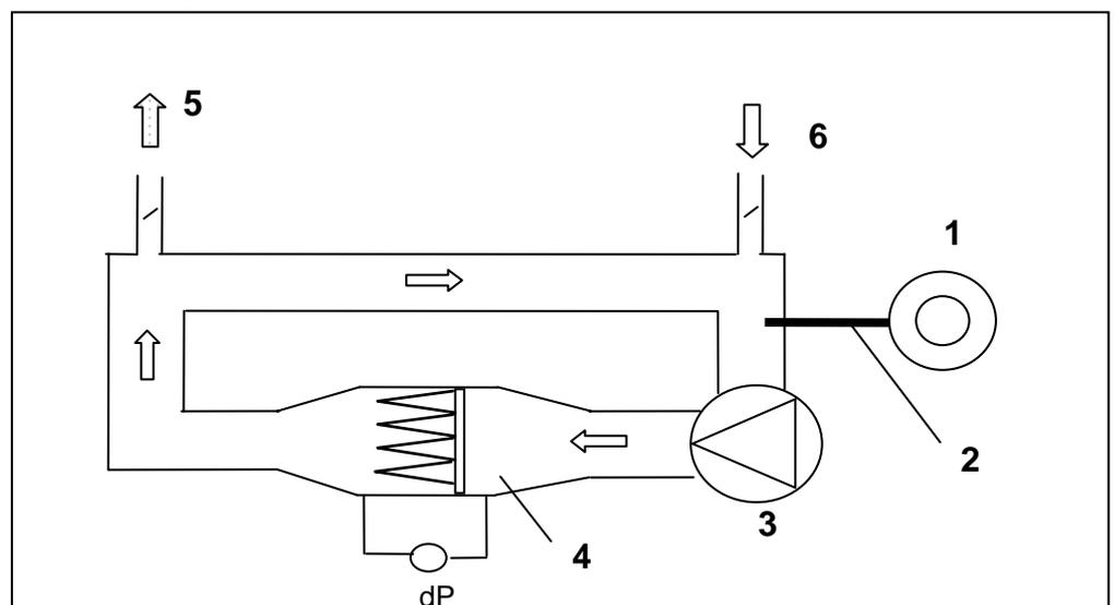
Figure 1 — Auxiliary test rig for preconditioning of filters
