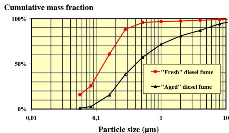
Figure 2 — Example of particle distribution from fresh and aged diesel fume (Lehtimäki 2006).
